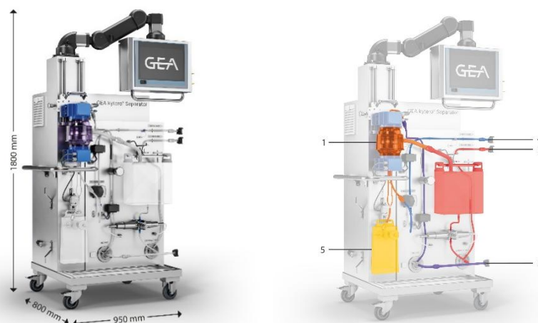
Figure 2-1: GEA kytero® 500 picture and schematic layout: (1) Separating unit (bowl); (2) Cell suspension feed line; (3) effluent line of clear phase to harvest bulk; (4) effluent line of solid phase / cell mass; (5) post production drain bag.
