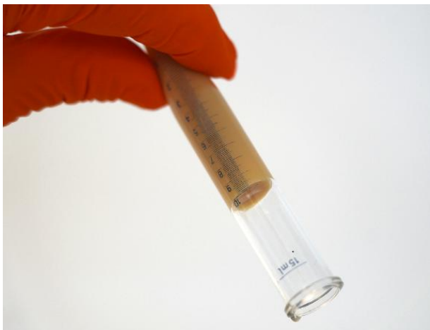
Figure 3-2: Exemplary picture of concentrate sample at setting of 50L/h and 7000 RPM with a stable cell pellet and no detectable residual fluid.
